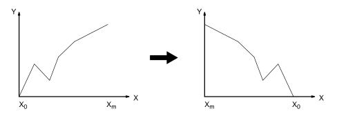
The following example demonstrates the construction of a linear approximation with 12 line segments. The block of data is continuous, as it must be, from DM 0000 to DM 0026 (C to C +  $(2 \times 12 + 2)$ ). The input data is taken from IR 010, and the result is output to IR 011.
